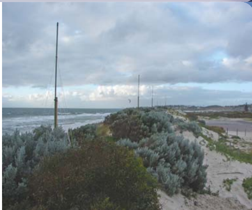
▲ Small receive antennae (3 m pole) linear array at Fremantle, Australia Range > 200 km
