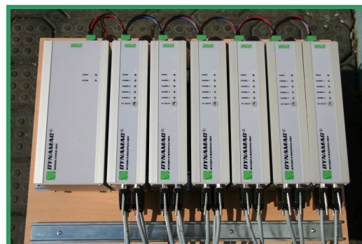
The set 1 NT800 + 6 MPX804R is designed for the measurement of 72 sensors
